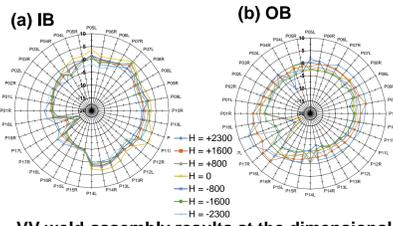
VV weld-assembly results at the dimensional error at sector generatrix
