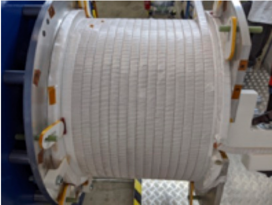
Figure 1: Fig. 1: Production inner-PF coil with two of four layers fully wound.
