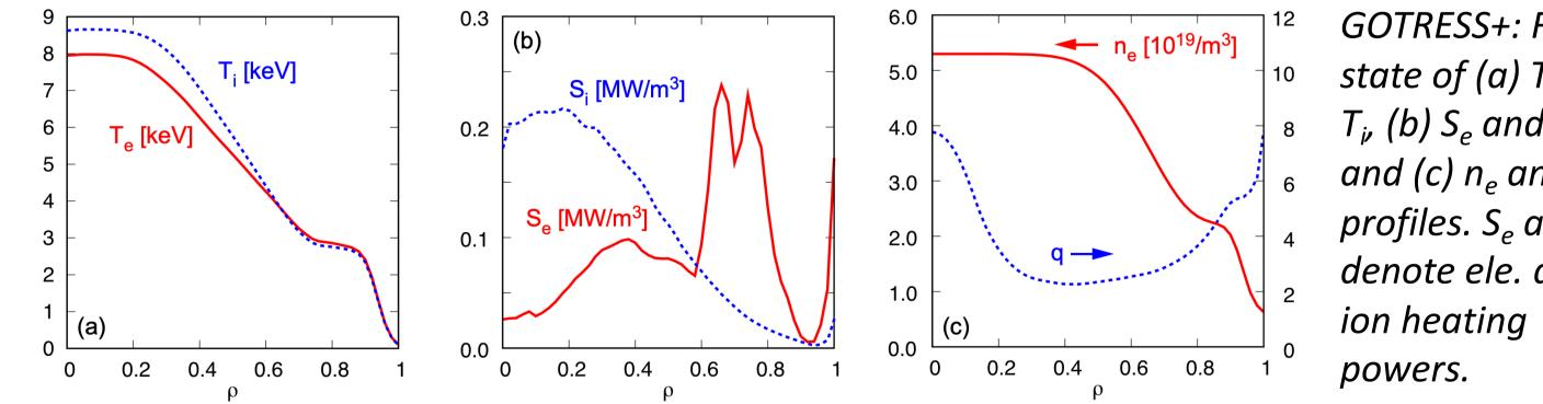
GOTRESS+: Final state of (a) T<sub>e</sub> and  $T_{i}$ , (b)  $S_e$  and  $S_i$ , and (c) n<sub>e</sub> and q profiles.  $S_e$  and  $S_i$ denote ele. and
