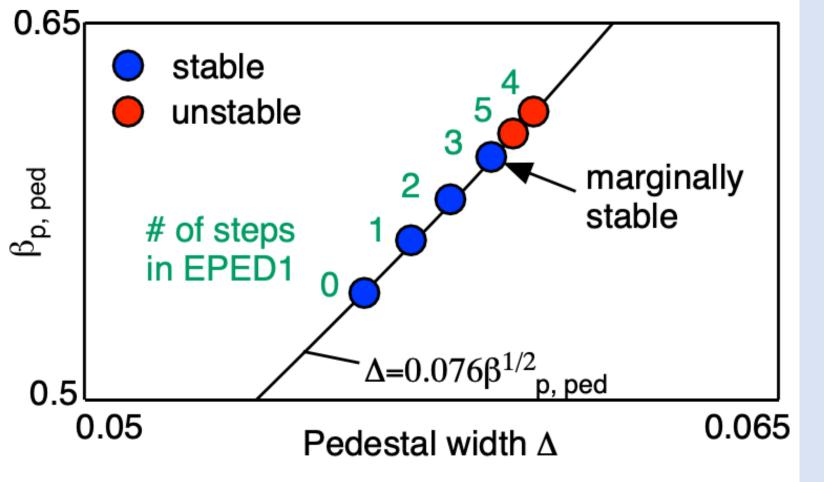
*Procedure in our EPED1 model to determine* the pedestal height in a marginally stable state
