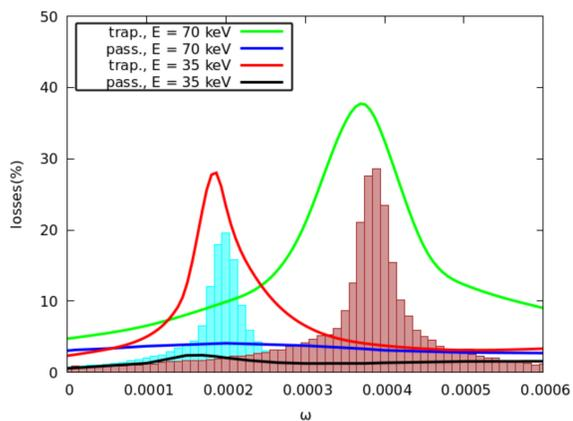
Ion losses vs NTM frequency. The histogram bars show the toroidal precession frequency of the trapped particles of 35 keV (cyan) and 70 keV (light red). When the frequency of the NTM matches the toroidal precession frequency of the trapped particles the losses increase significantly. The losses of passing particles show a mild dependence on the NTM frequency.
