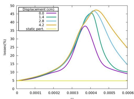
Ion Losses vs NTM frequency when  $B_1$  and  $E_1$  are on. The electric field of the NTM transfers energy to the particles increasing their average precession frequency.
