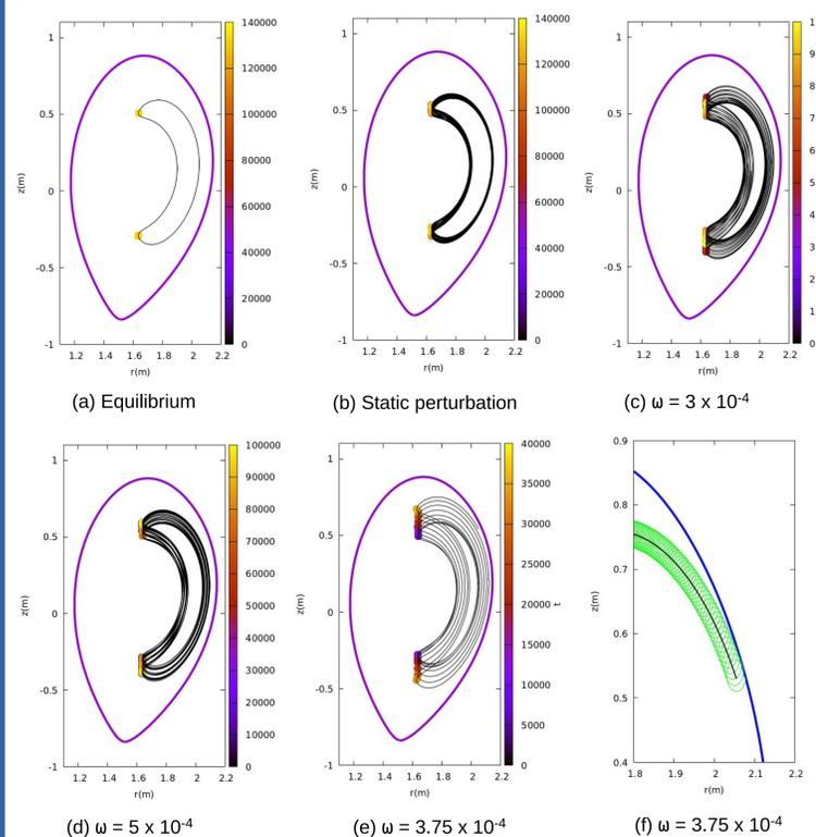
When  $\omega = 3.75 \times 10^{-4}$  frame (e) the particle is lost. The colored point indicates the bouncing position and the color scale is time. LFCS is in blue. In (f), the full orbit (green line) touches the LFCS but the GC orbit (black line) doesn't.
