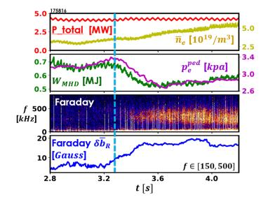
Figure 1: Magnetic turbulence is observed to correlate with confinement degradation during density ramp in ELMy H-mode
