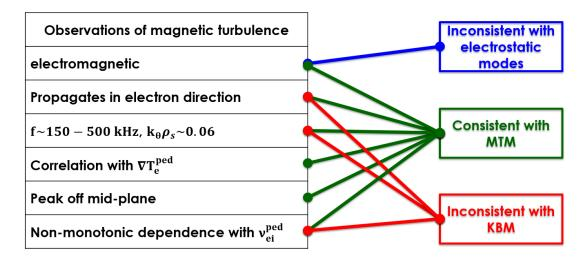
Figure 2: Identification of observed magnetic turbulence in ELMy H-mode plasmas
