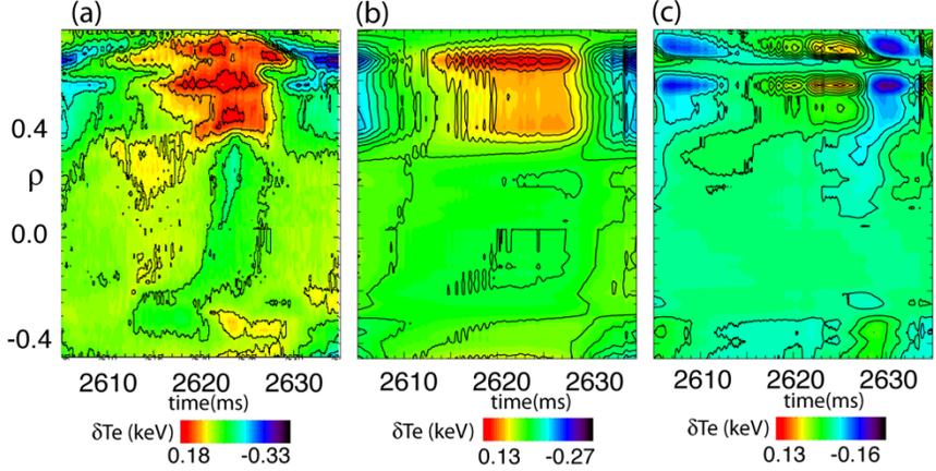
Fig. 9. The QI-driven crash hand-shaking with outer  $n=1$  and  $n=2$  reconstructed components. (a) the  $d\text{Te}$  contour by ECE profile, the reconstructed (b)  $n=1$  component and (c) the  $n=2$  component.
