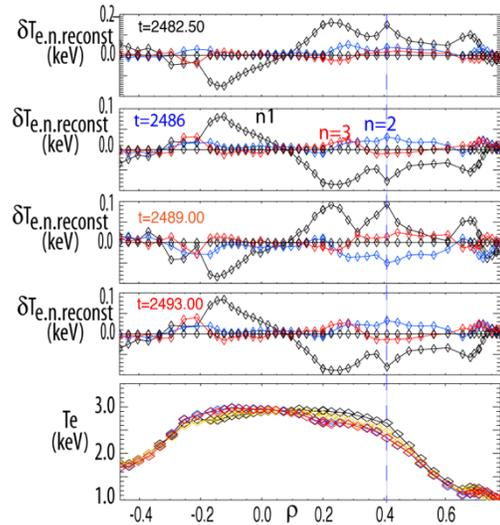
Fig. 6. The radial structure of  $\delta T_{n.reconst}$  profiles of the components,  $n=1$  (black),  $n=2$  (Blue),  $n=3$  (red). Time slices are 2482.50ms, 2486ms, 2489ms and 2493ms. The profile at the bottom are total components added at 2482.5ms (Black), 2486ms (Blue), 2489ms (Orange) and 2489ms (red)
