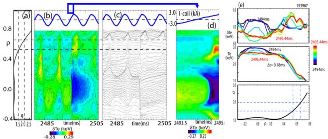
Fig.4. The formation of Te collapse. (a)  $q$  vs  $\delta$ , (b) the  $\delta Te$  contour (c) the  $\delta Te$  vs time (d) the expanded Te collapse and (e) the  $\delta Te$  crash details and Te profile(top) and  $dTe$ (middle) vs  $\rho$ -radius at various time slices,  $t=2594\text{ms}$ (blue), and  $=2495.44\text{ms}$  and with every  $144\mu\text{s}$  interval), The blue curves in Fig.(b,c,d) are I-coil current and  $q$  vs.  $\rho$  (#153967).
