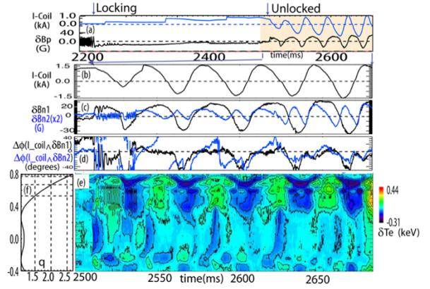
Fig. 7. QI mode under tearing mode locking avoidance: (a) I-coil current and magnetic signal, (b) I-coil current, and magnetic sensor signal amplitude with decomposition,  $n=1$ ,  $n=2(x2)$  (d) the phase difference between the external field and  $n=1$  (black) and  $n=2$  (blue) component, (e) the contour of  $dTe$ , and (f)  $\rho$  vs.  $q$  (#153974)
