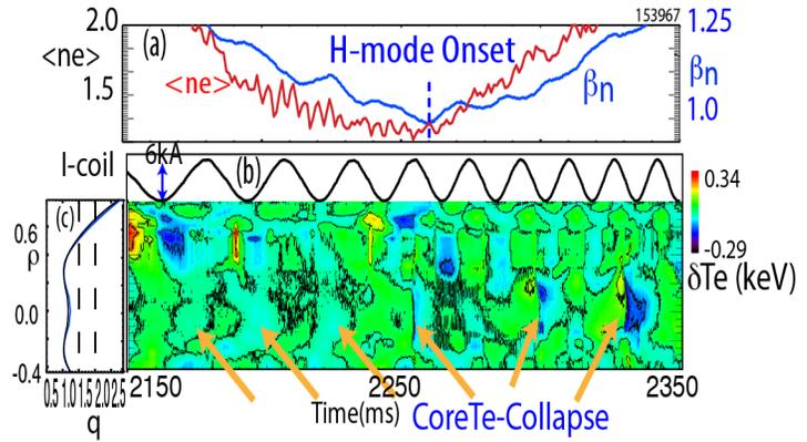
Fig. 3. The Core-Te-collapse behavior around H-mod onset (#153967) (a) The electron density and beta-n,  $\beta_n$ , (b) I-coil current and the perturbed  $dTe$  (c) the  $q$ -profile( $x$ -axis) vs.  $\rho$ ( $y$ -axis)
