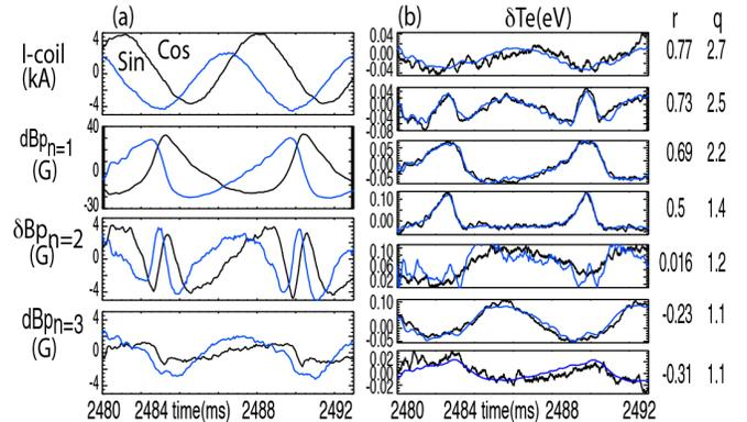
Fig. 5. The magnetic sensor input signals to determine the reconstructed  $\delta Te$  (#153967): (a) from the top, I-coil,  $n=1$ ,  $n=2, n=3$  components. (b) comparison of the fitting between the ECE signals (black) and the reconstructed  $\delta Te$  (blue)
