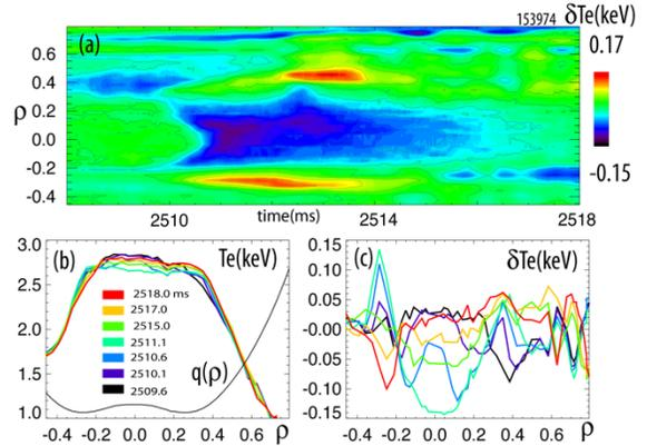
Fig. 8. The QI-crash structure at  $t=2510$ ms. (a)  $\delta Te$  time development, (b)  $Te$ -profile and (c)  $\delta Te$  at various times
