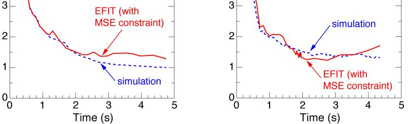
Strong off-axis current drive results in higher q<sub>min</sub> than usual for hybrid scenario
