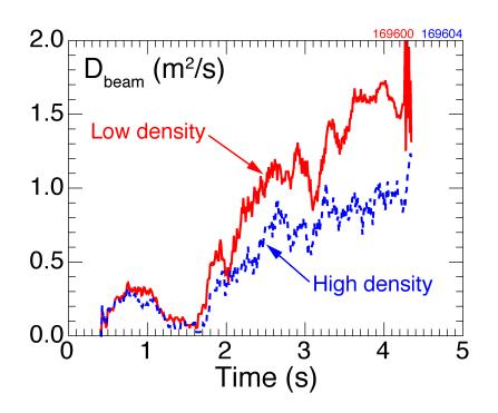
Lower D<sub>beam</sub> at higher n<sub>e</sub> is consistent with weaker toroidal Alfvén eigenmode activity
