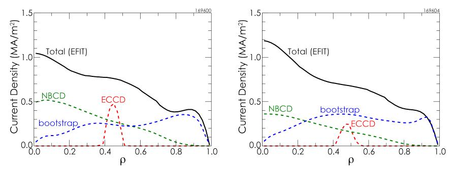
Bootstrap current fraction is unchanged between low and high density hybrids
