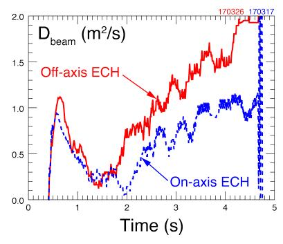
Larger D<sub>beam</sub> for off-axis ECCD is consistent with stronger toroidal AE activity above 100 kHz
