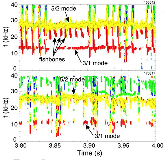
Steady-state hybrids with on-axis ECCD and q<sub>min</sub>≈ 1 generate strong fishbones
