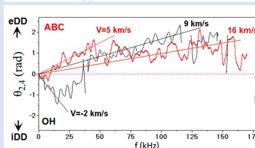
The cross-phase of density fluctuations vs frequency for OH (black curve) and ABC (red curve) stages of the shot with changes of the potential sign #73197;  $B_t = 2.2$  T,  $I_{pl} = 230$  kA,  $E_b = 320$  keV,  $r_{HIBP} = 0.09-0.11$  m.
