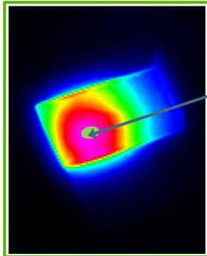
Laser spot dimensions ( $\sim 4 \times 2$  mm)
