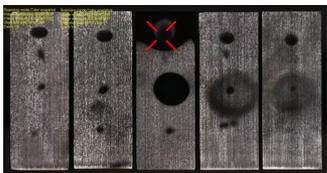
Fuzzy ring grown with thickest coverage around 3 mm from beam centre
