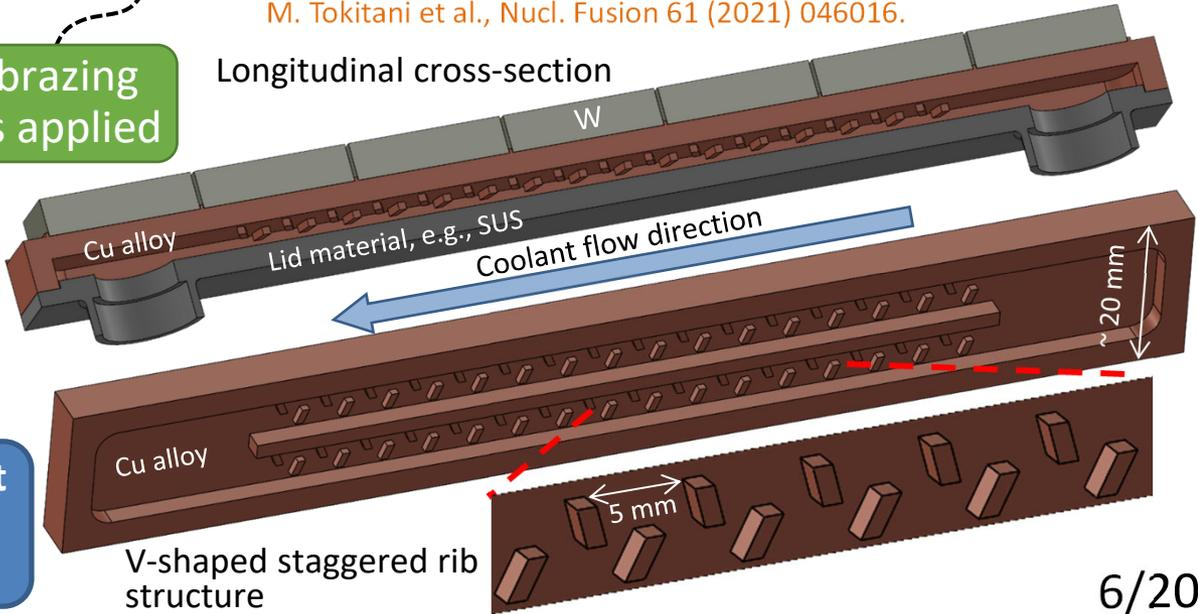
The leak-tight joint is difficult to create in the conventional technologies.
