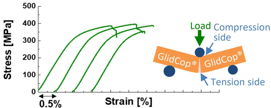
(a) Three-point bending test
