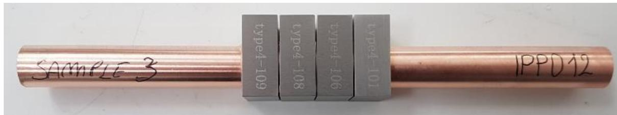
brazed joint between W mono-blocks and  $W_f$  - Cu heat sink pipe
