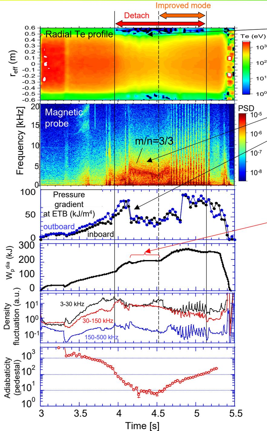
As the detachment deepens, the edge  $T_e$  decreases due to impurity radiation → resistivity increases
