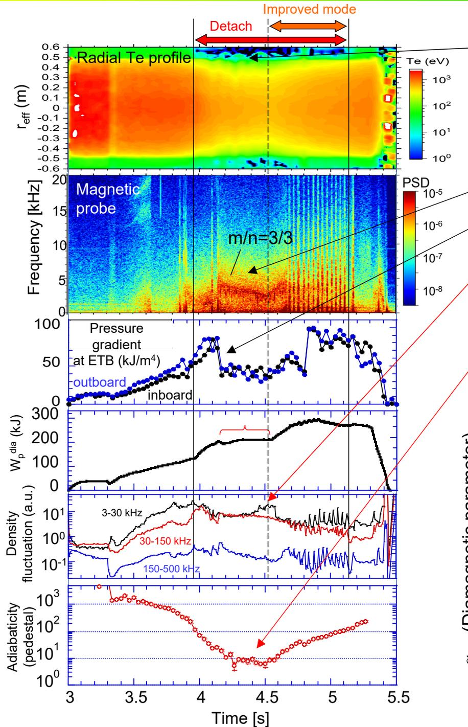
As the detachment deepens, the edge  $T_e$  decreases due to impurity radiation → resistivity increases
