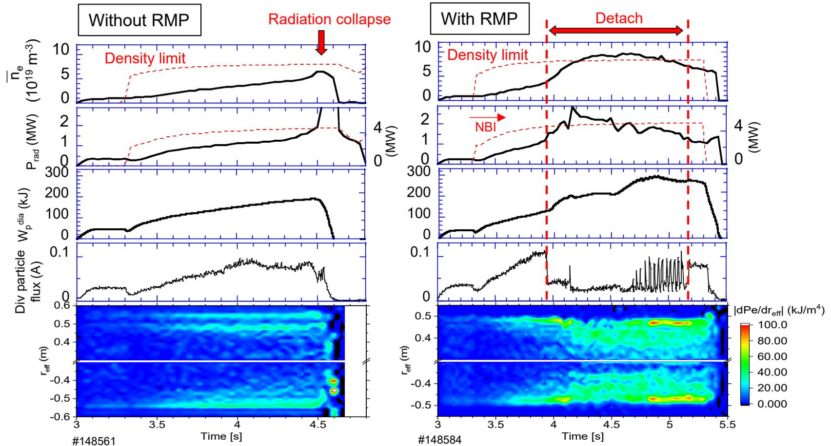
Change of edge magnetic field structure/topology resulted in significant difference in core and divertor performance.
