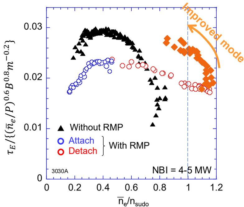
Confinement sustained at higher density with RMP application ← Due to ETB formation
