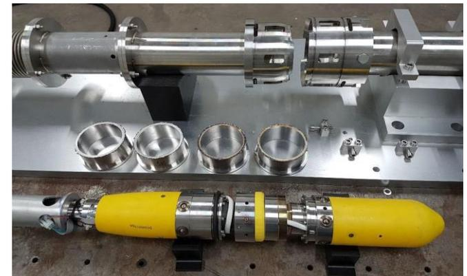
*In-bore cutting tool and test rig*
