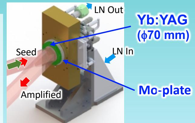
Reduced-stress active-mirror at 77K using original bonding technology
