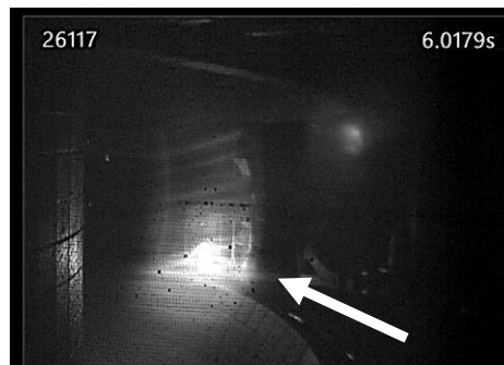
Fig. 11. Example of Oport fast camera view of the SPI fragment interaction with the plasma. The arrow shows the shattered pellet trajectory with the inner wall on the left.
