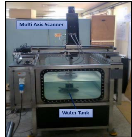
Facility for performing Immersion UT examination at IPR
