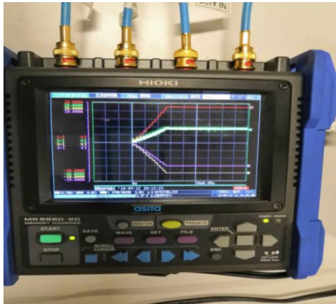
1 st STEP 1200kV-1 HOUR
