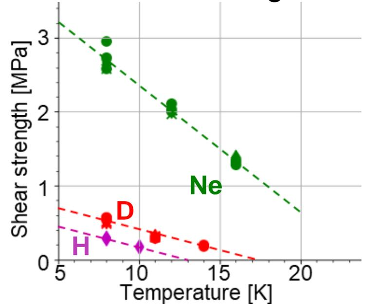
**Shear strength depends on pellet material and decreases with increasing temperature**
