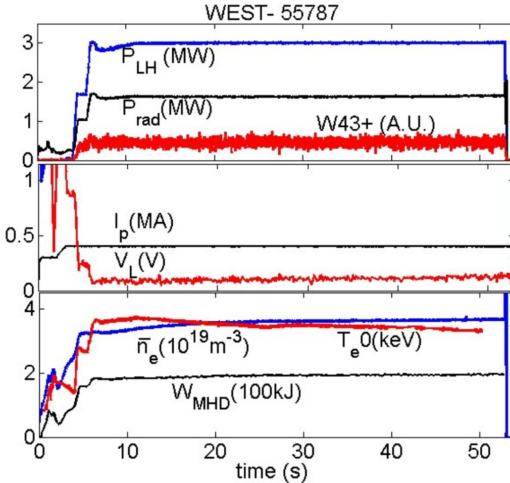
Figure 2: 53s-long discharge ( $B_t/I_p=3.7T/0.4MA$ , USN configuration)
