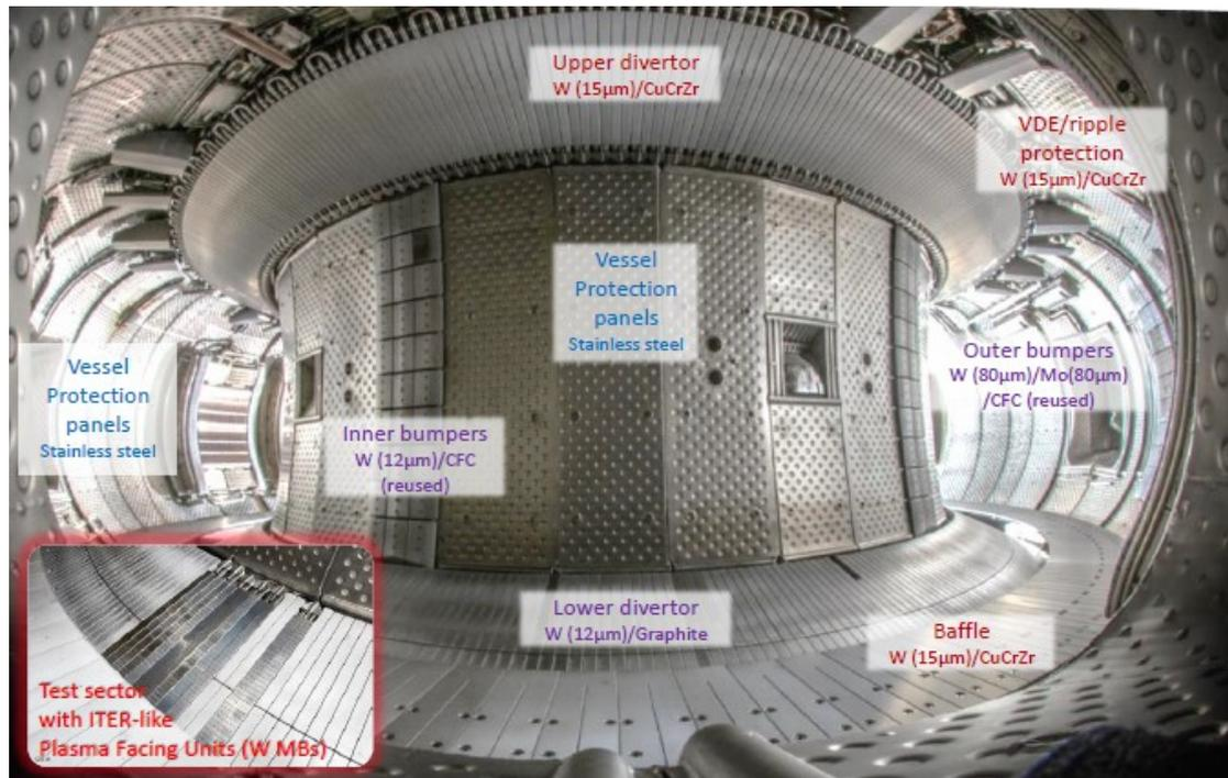
Figure 1: Picture of WEST vacuum vessel, May 2018
