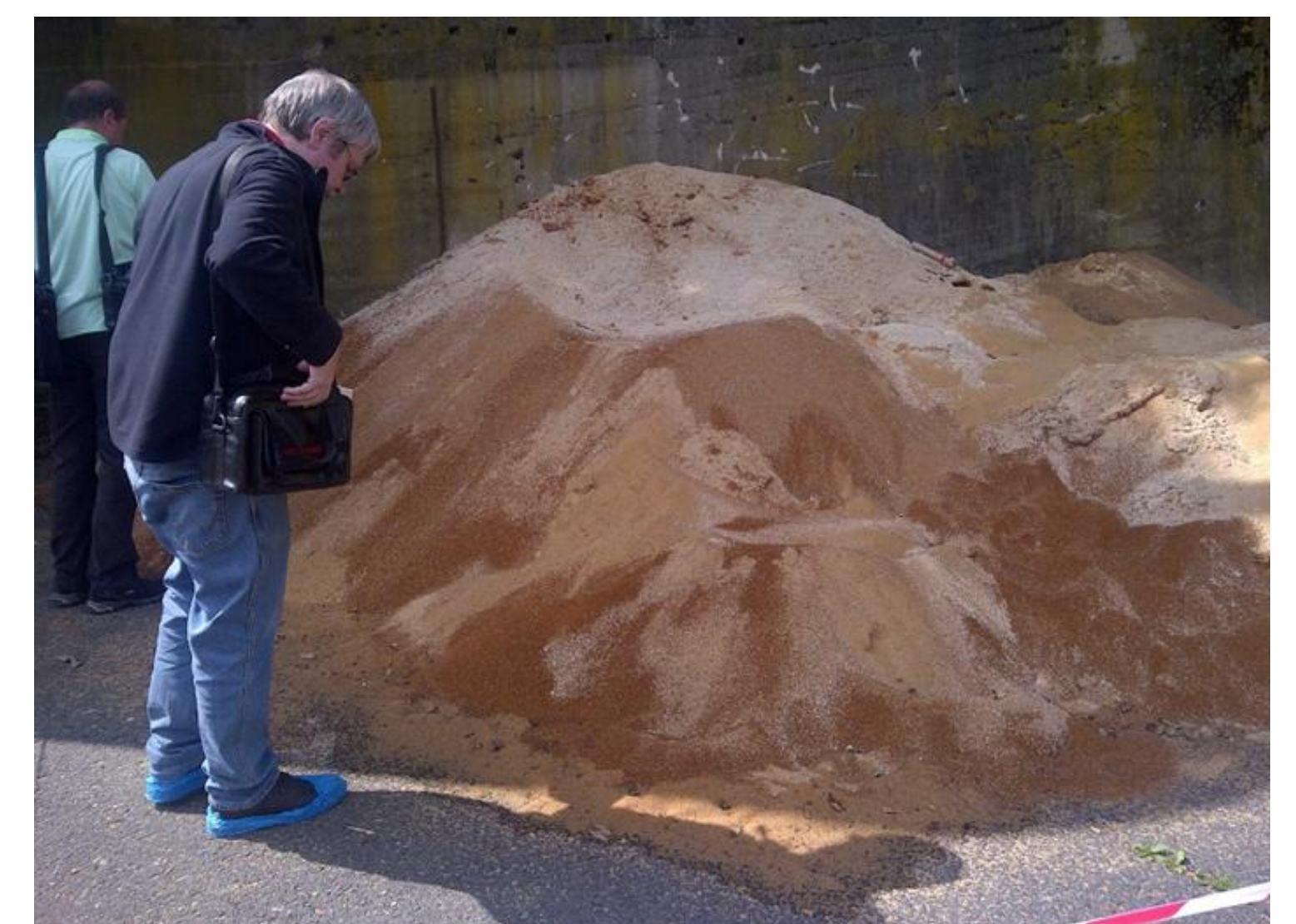
FIG. 2. NORM materials – sand from the water treatment plant of the public swimming pool
