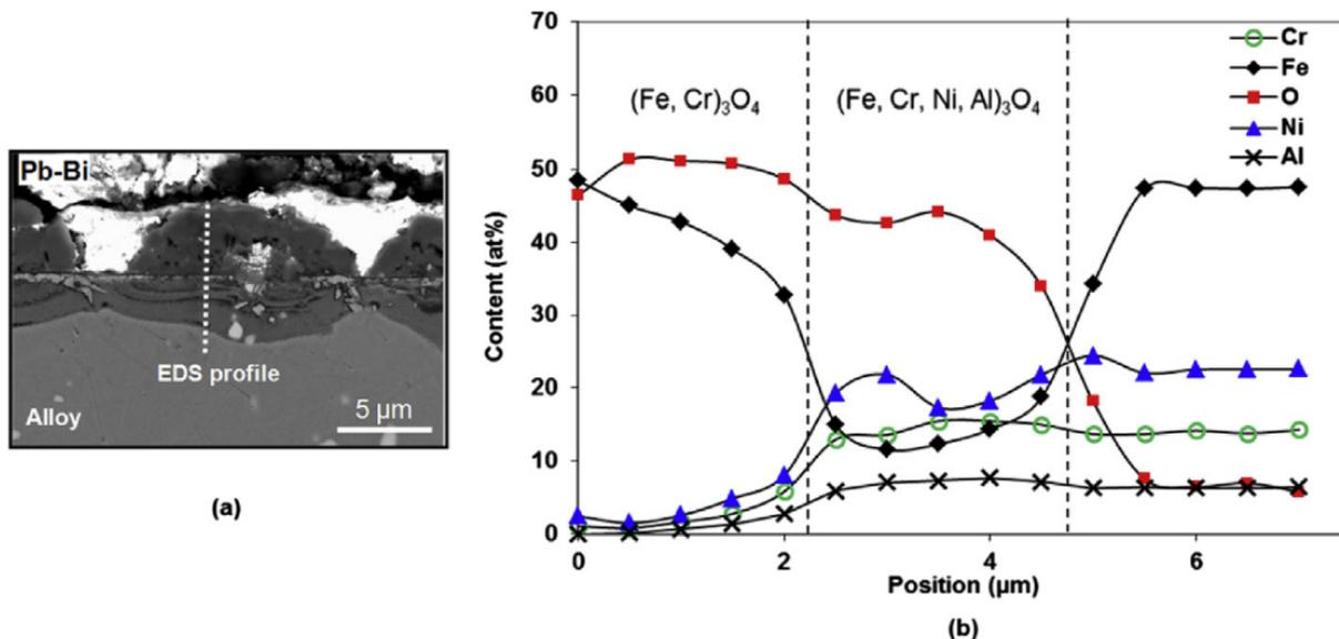
SEM Photograph of polished cross section of OC-4 material after immersed in LBE for 190 h at 520 °C [1]
