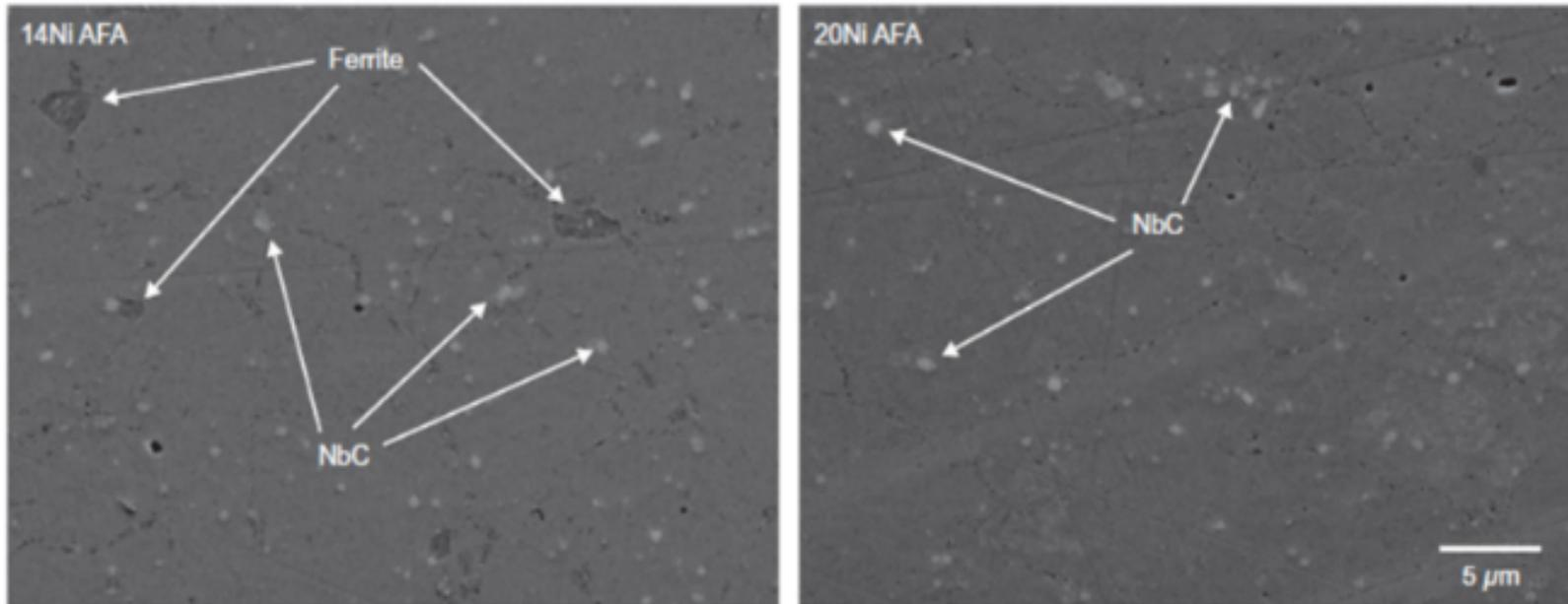
NbC particles with secondary phase, ferrite, in 14Ni AFA steel
