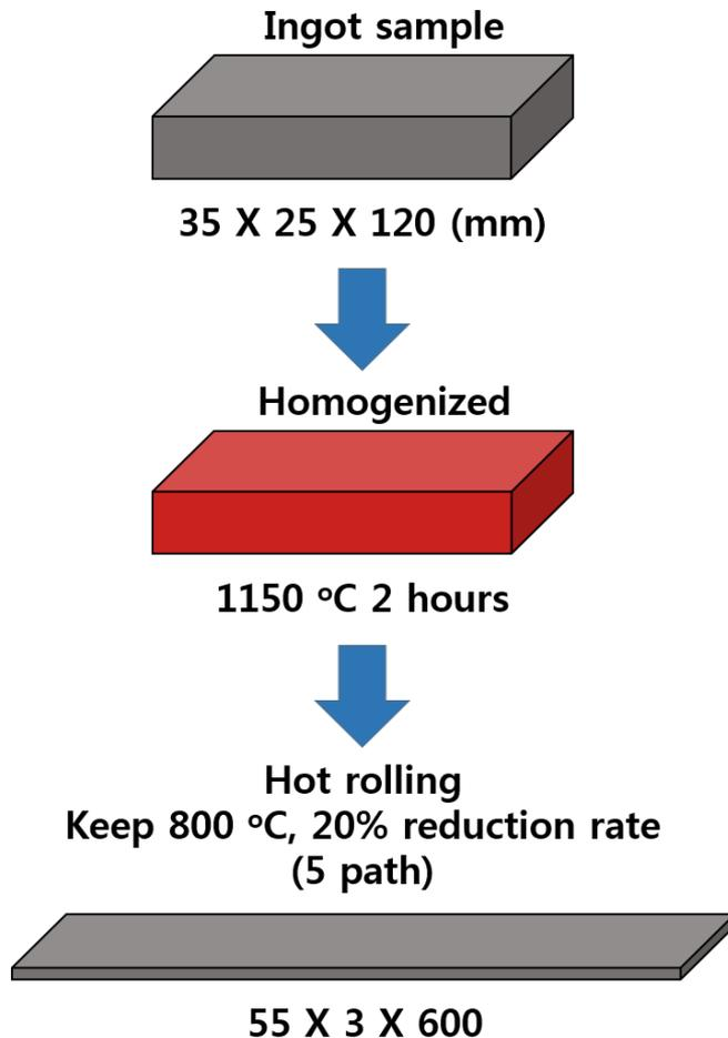
Fig. Process schematic ( Width X thickness X length)
