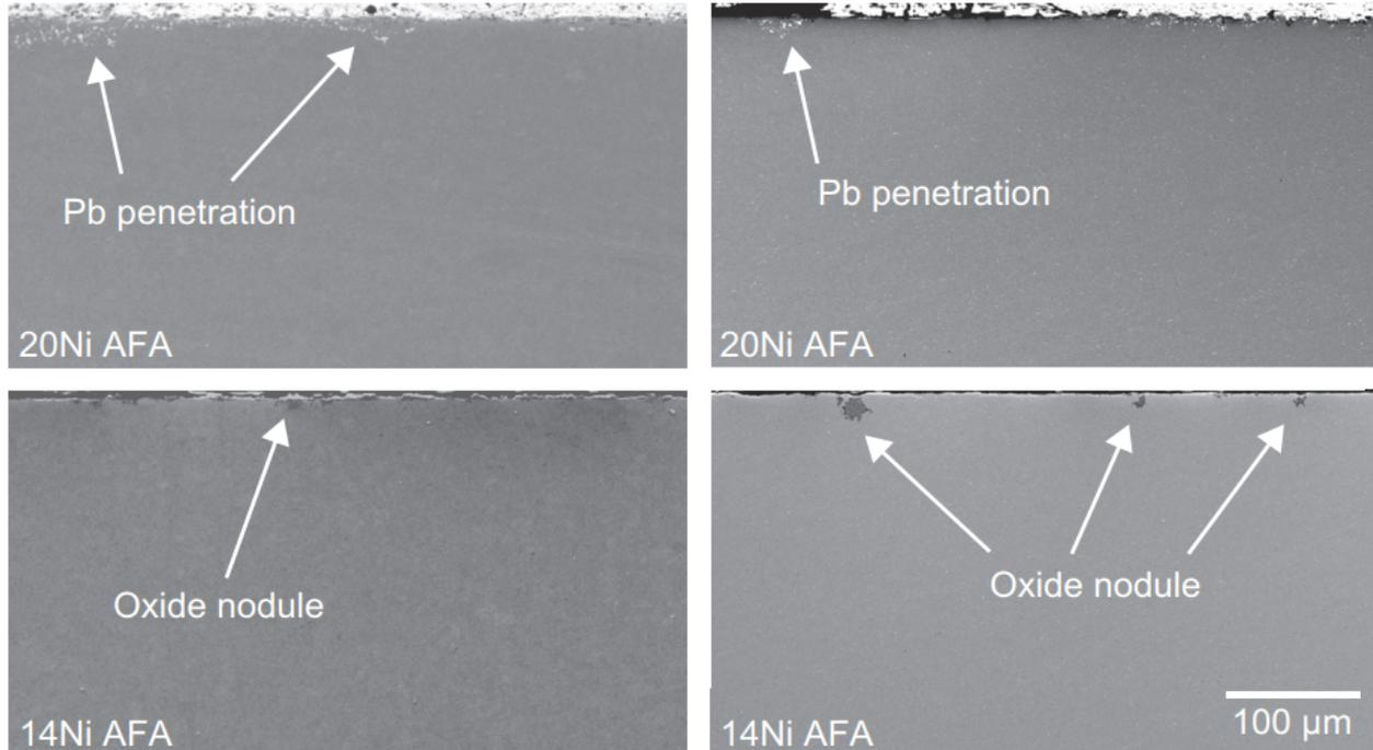
Cross section images of the materials exposed in Pb for 3,000 h (left) and 8,760 h (right) at 550 °C
