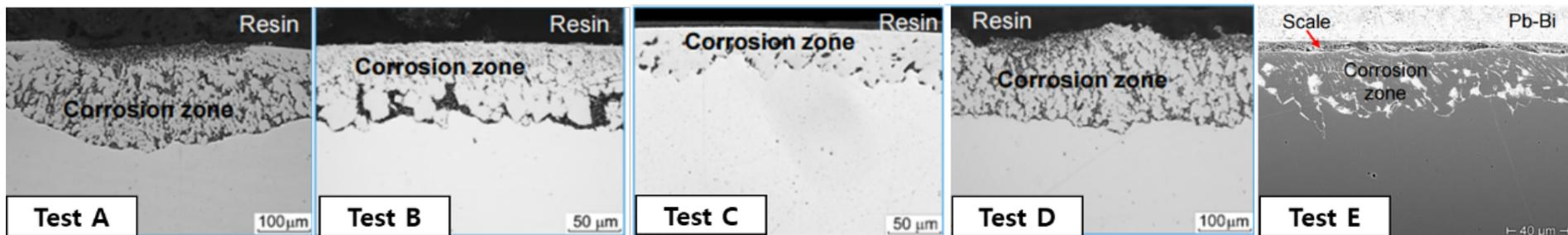
Corrosion test results of #3-AI depending on dissolved oxygen concentration
