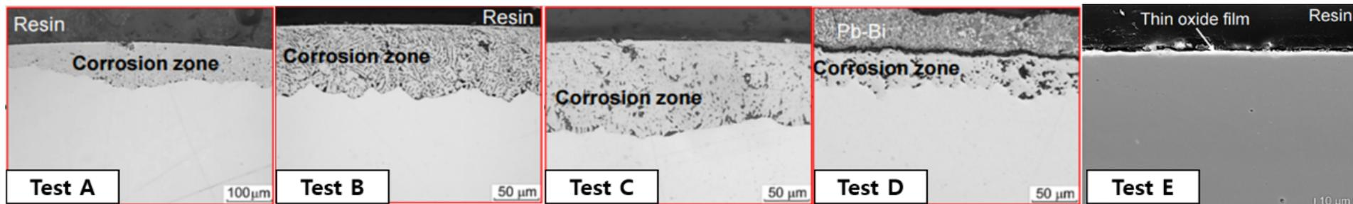
Corrosion test results of #1-AINbC depending on dissolved oxygen
