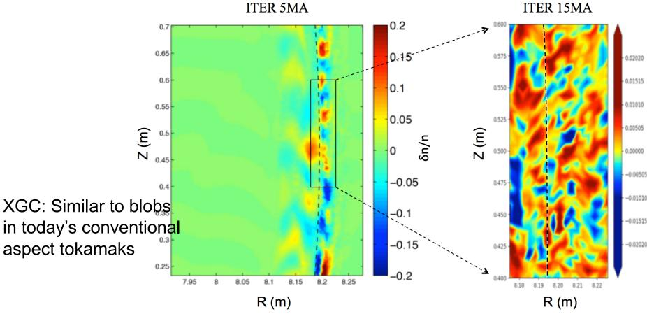
TEM streamers are the suspect. ITGs do not penetrated into SOL [Chang, 2009].
