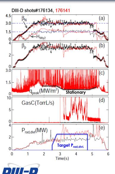
> Feedback control of  $\beta$  & divertor radiation simultaneously.
