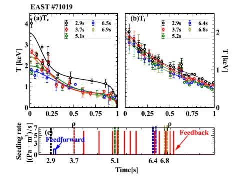
Total radiation fraction can be flexibly controlled within 18-36%, in H-mode regime. f<sub>rad</sub> extended to 41% in 2018.
