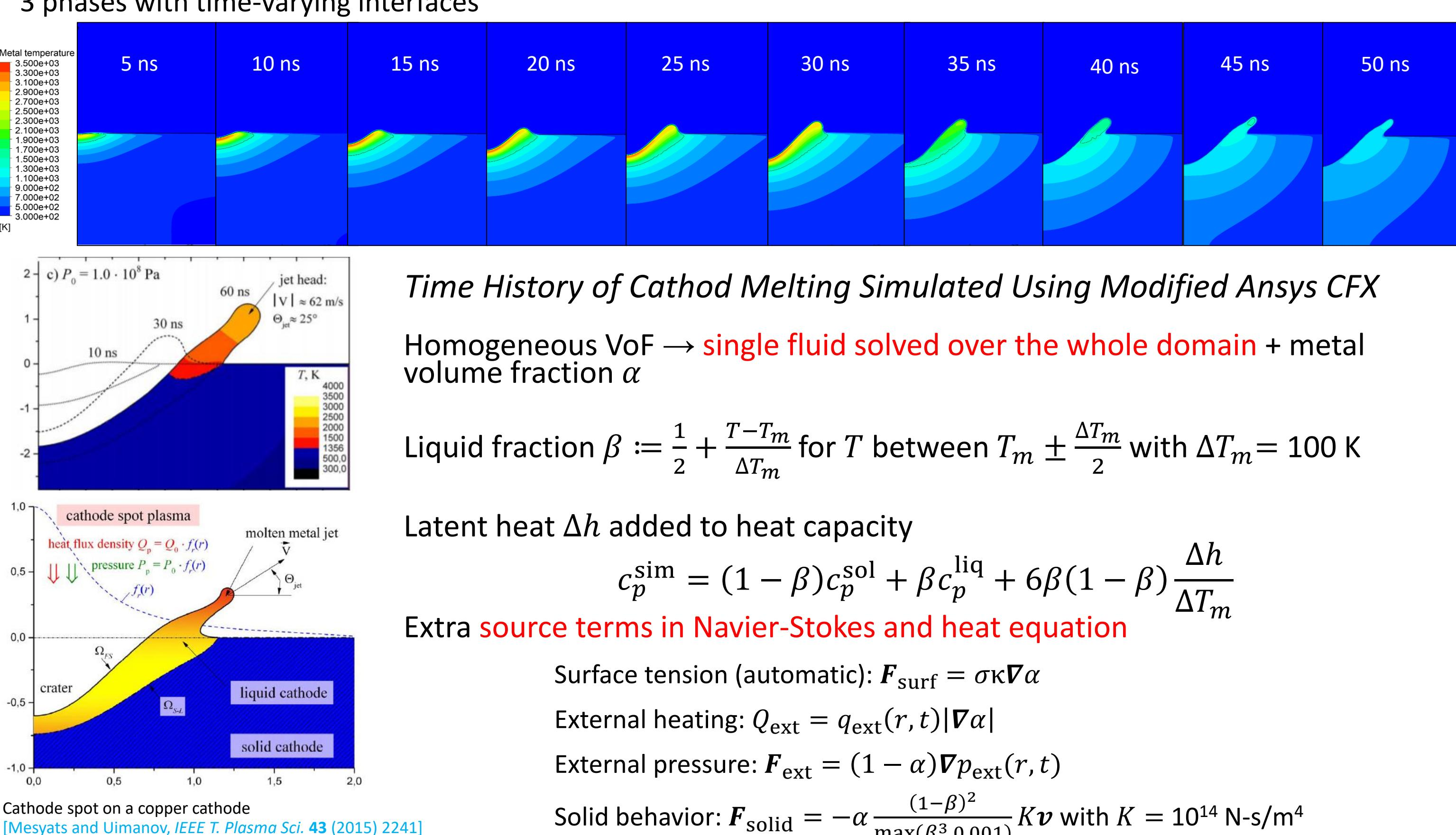
Time History of Cathod Melting Simulated Using Modified Ansys CFX
