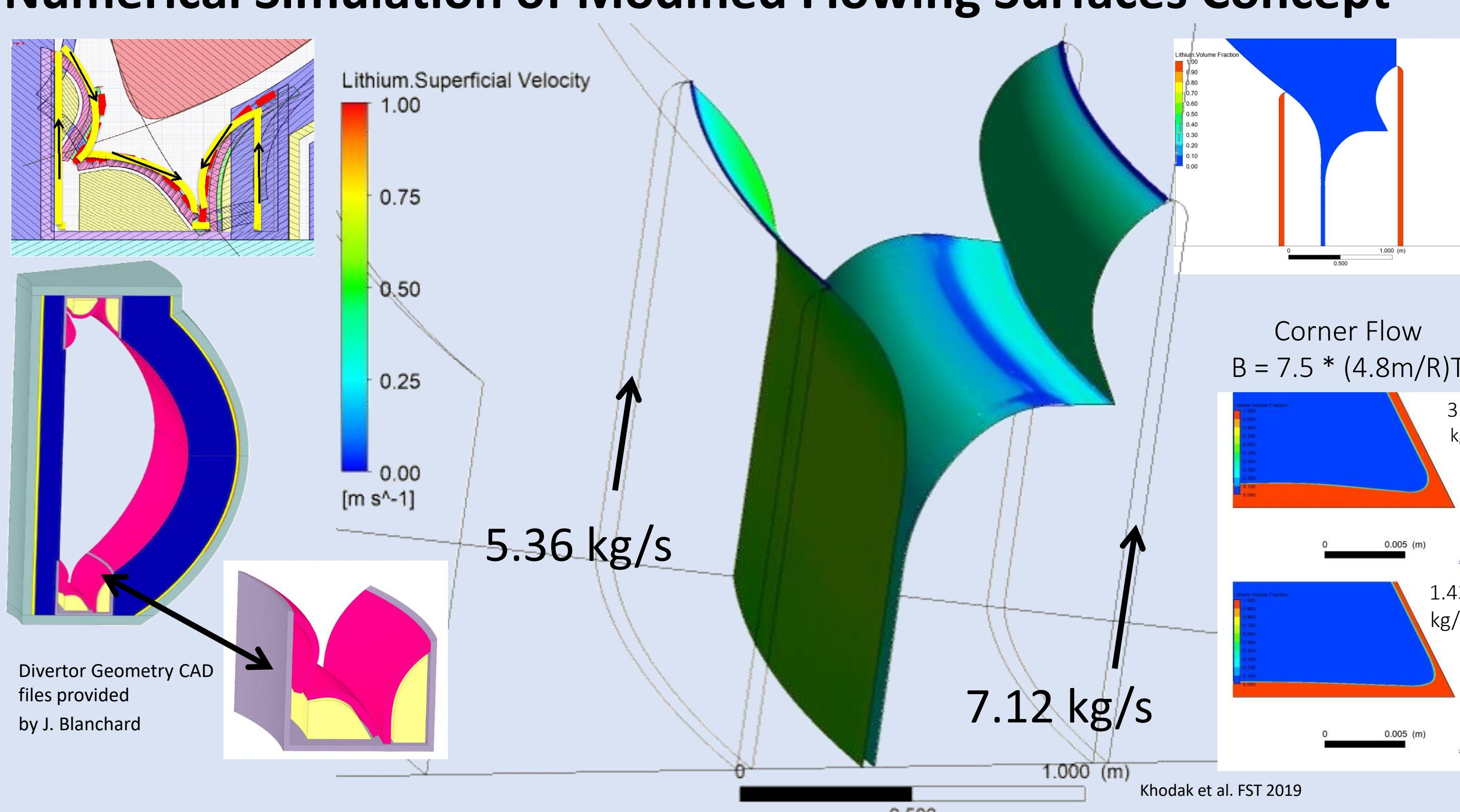
Numerical simulation of the liquid lithium free-surface cooling system for future fusion device design developed for FNSF program. Design includes LM PFC covering convex diverter surfaces, as well as lithium supply and removal lines.
