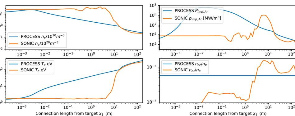
The calculated power crossing the separatrix is in good agreement, as well as the boundary conditions at the target and the midplane. SOL behaviour near the target is not accurately captured in the 1D code because of uncaptured physical processes, such as radial transport near the target, and a fixed argon density, however the purpose of the 1D code is to accurately model detachment conditions and estimate  $P_{sep}$ .
