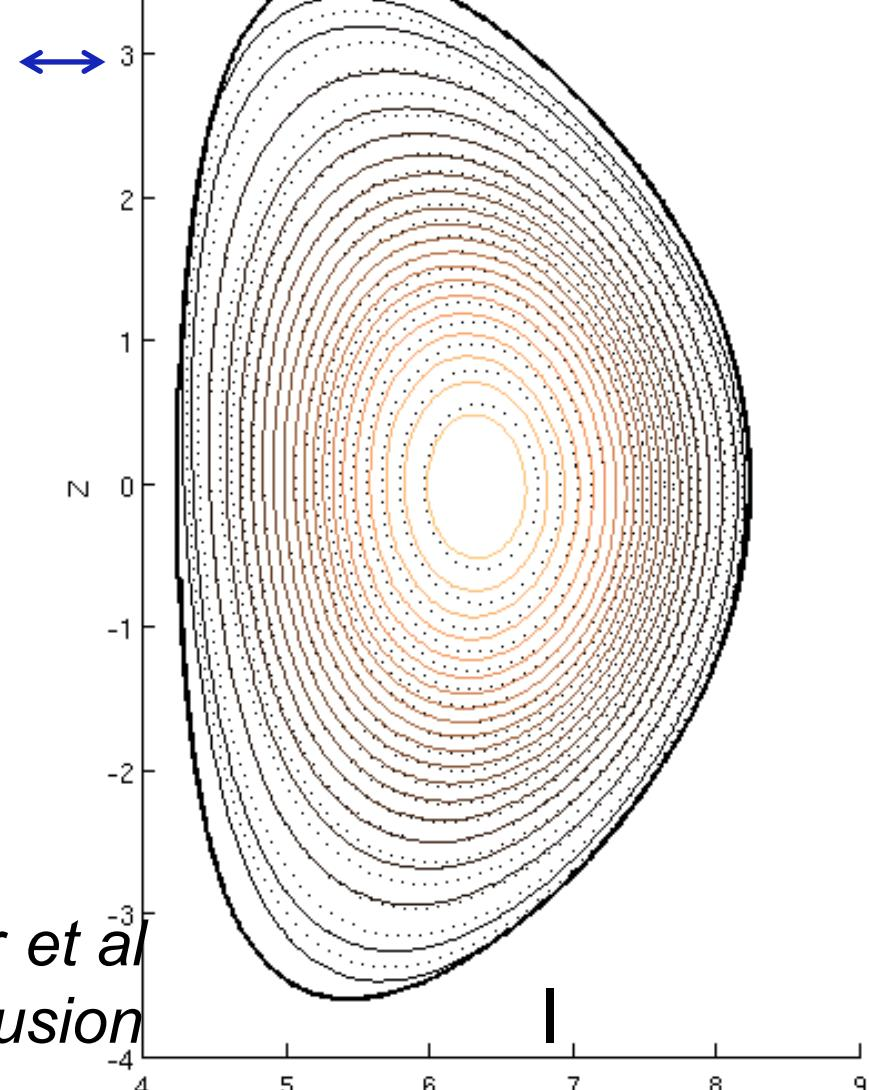
Shift from magnetic axis  $\propto$  anisotropy
