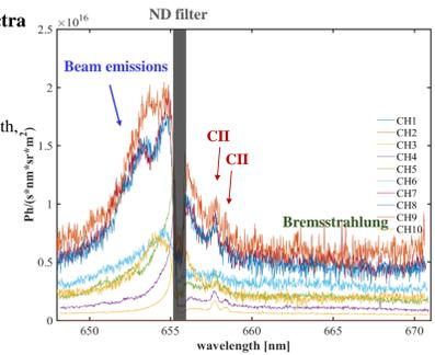
Non-charge exchange component (OV, CII, OIV...) can be subtracted by beam modulations.
