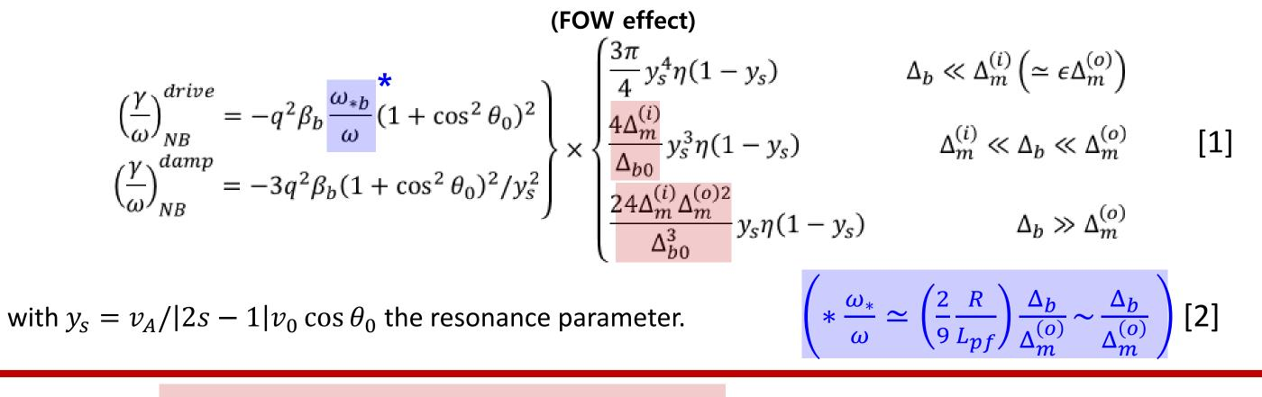
$\gamma/\omega$  has different scaling dependence of  $\Delta_b/\Delta_m$  w.r.t the orbit width regime [1].
