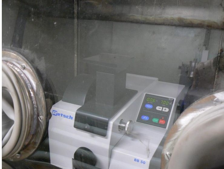
Fig. 3. Newly installed Retsch BB 50 Jaw Crusher
