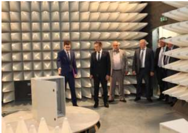
Semi-anechoic chamber for the EMC compatibility testing
