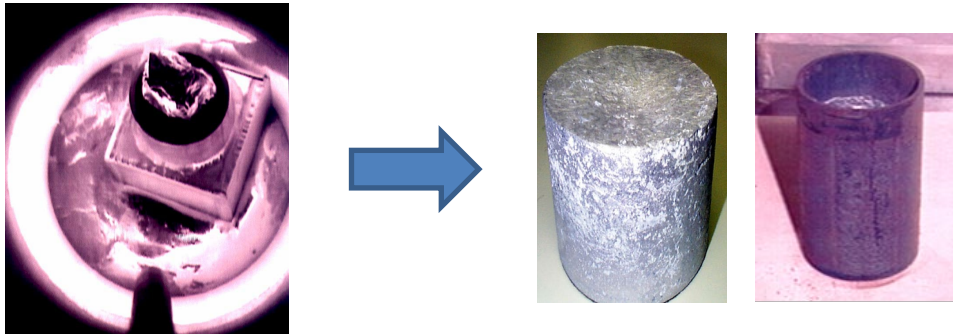
FIG. 4 Melting fuel element and final fuel form.
