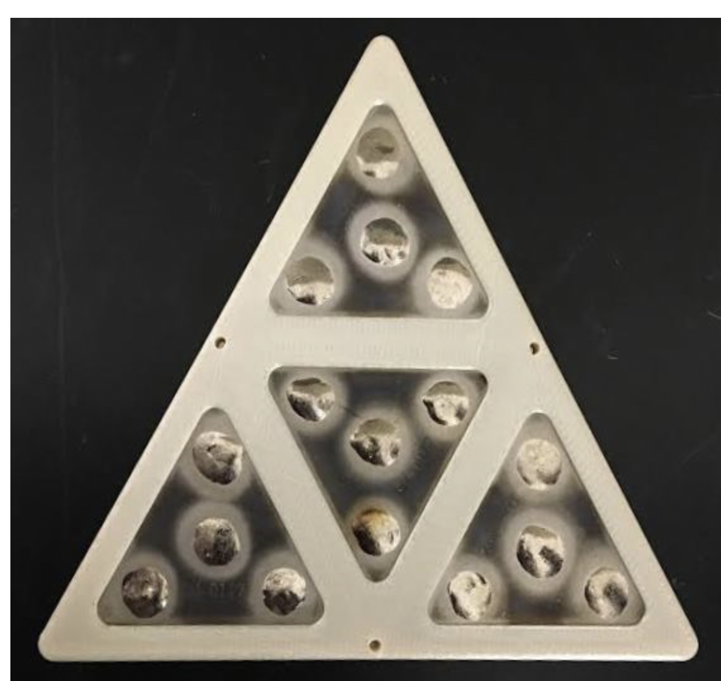
Figure 2. Plastic frame subassembly of four RSTD sources.
