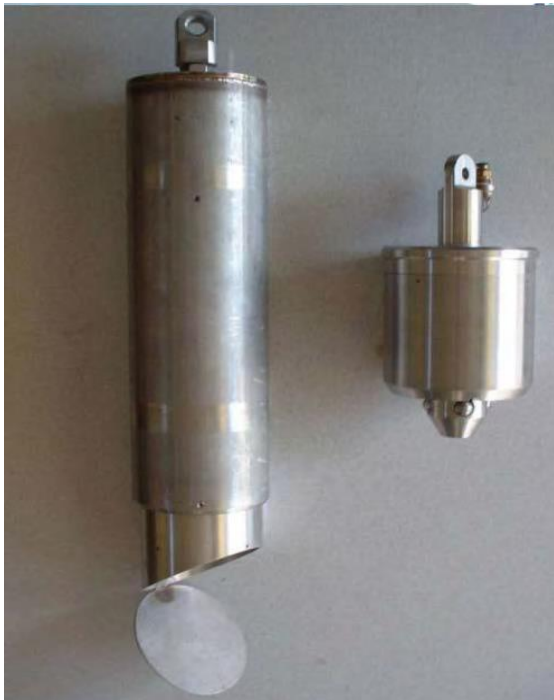
Figure 4: Cement Dumping Container (Hooper) and Pneumatic Grabber
