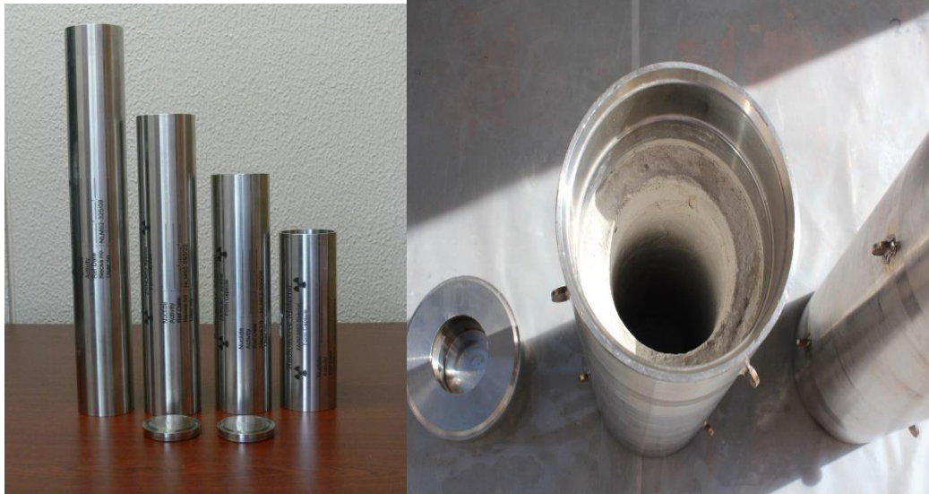
Figure 3. (a) Stainless-steel capsule; (b) cement-based containment barrier inside the stainless-steel disposal containers
