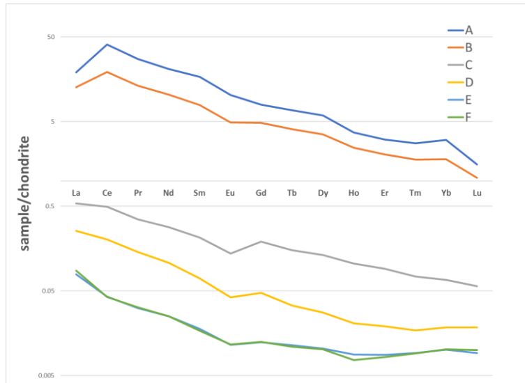
FIG. 11. Diagram of the rare earth elements (REE) for all UOC samples by ICP-MS (data LLNL). The chondrites were normalized using the mid ocean rich basalt (MORB) values from Pierce (1973) and Bevins (1984).
