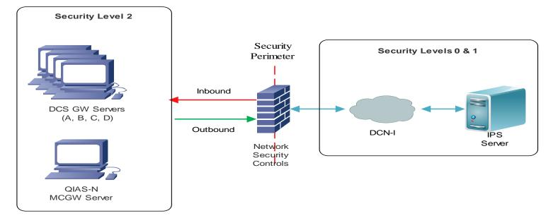
Establishing a computer security perimeter as an FPGAbased network security controller between the DCN-I Subnet and DCS safety-channel gateway servers Subnet is to implement security controls for controlling and managing the inbound data traffic.
