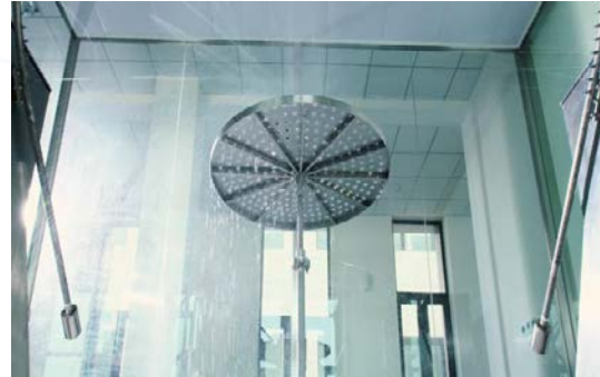
Water Proofing Test System
