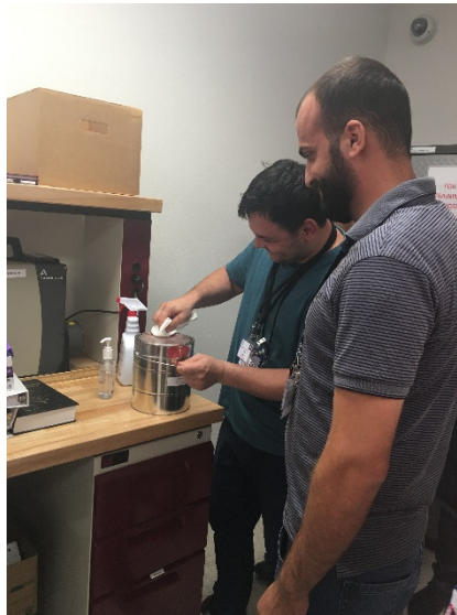
Fig. 1. Participants Constantin Sumanariu (L) and Alaaddin Alnajjar remove TID adhesive residue (seen in red), from a container of nuclear material in preparation to apply a new TID.
