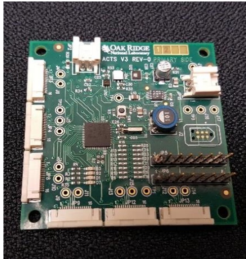
FIG. 4. The low-power ACTS circuitry with sensor suite and peripheral expansion slots extends capabilities, while the IMU senses motion to reduce power consumption and allow smarter control of the communication device's power.
