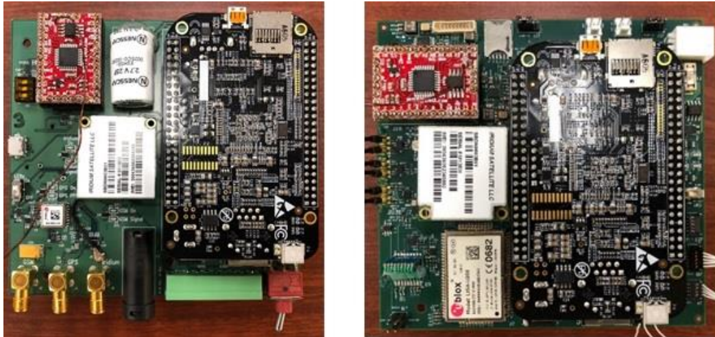
FIG. 3. Gen 2 variations can independently switch between two antennas for each radiofrequency device, control the GPS device's low-noise amplifier, and alter component placement to facilitate inserting the SD and SIM and routing enclosure cables.
