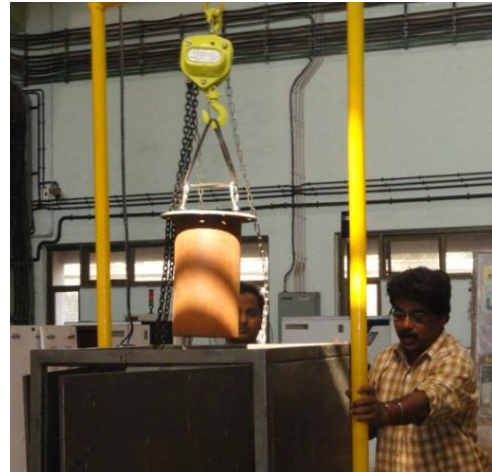
Fig. 2(b). Removing the cage plug
