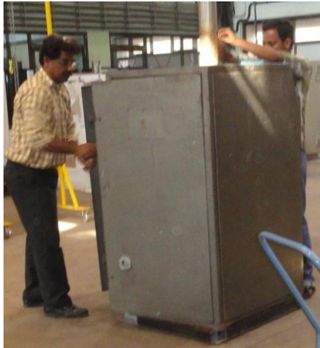
Fig. 2(a). Removal of outer cabinet
