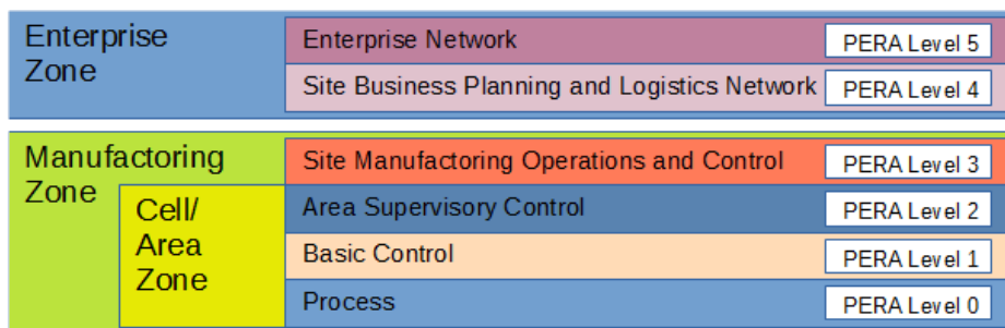
Fig. 1. Control Hierarchy of ICS according to [1]
