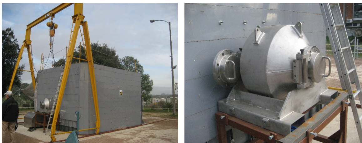
Figure 4. LTSS mated to mobile hot cell
