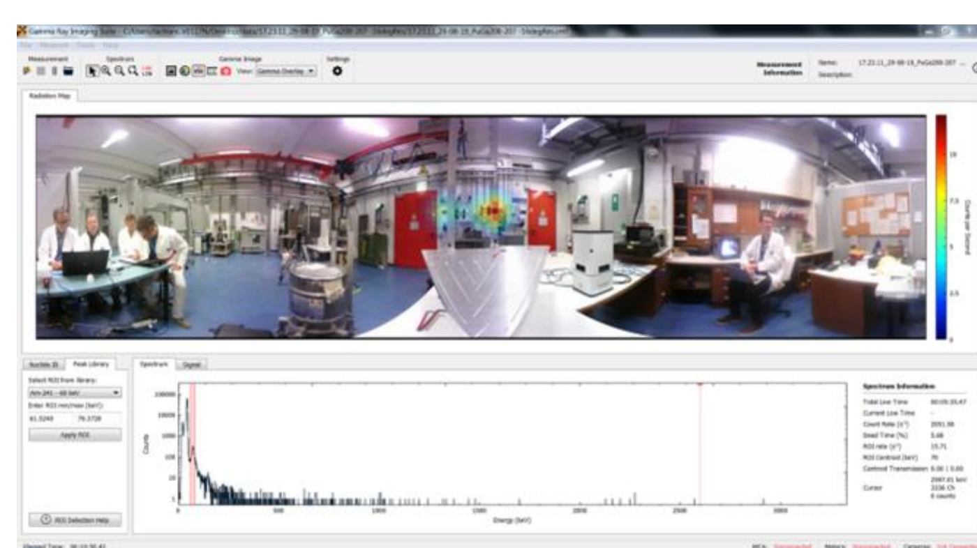
Angular resolution of 16^\circ measured on a test rig with non-infinitesimal sources size (2 PuGa discs) measured at the JRC-Ispra
