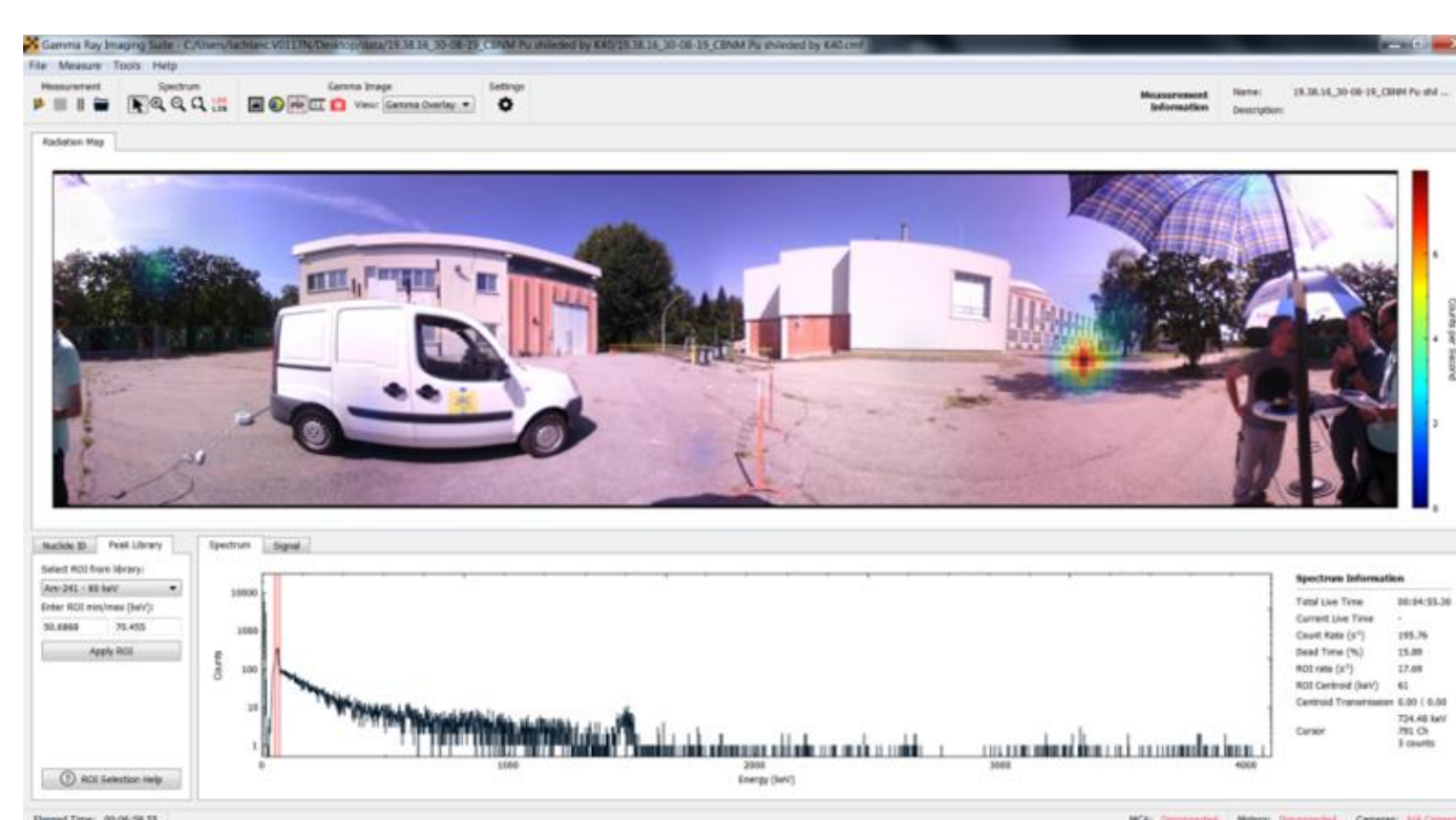
^{241}\text{Am} peak localized at distance of 23 m in a few minutes
