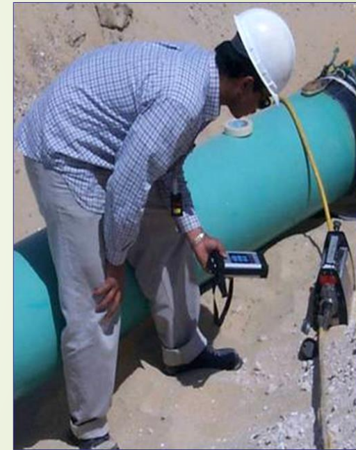
Industrial radiography of pipes using Iridium-192
