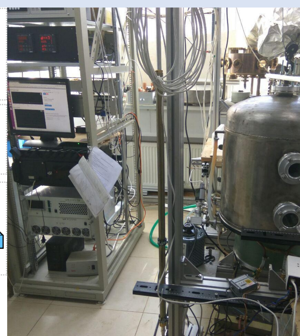
Fig. 6: Thermo-vacuum test Bench for research on RF-cables and in-vessel components
