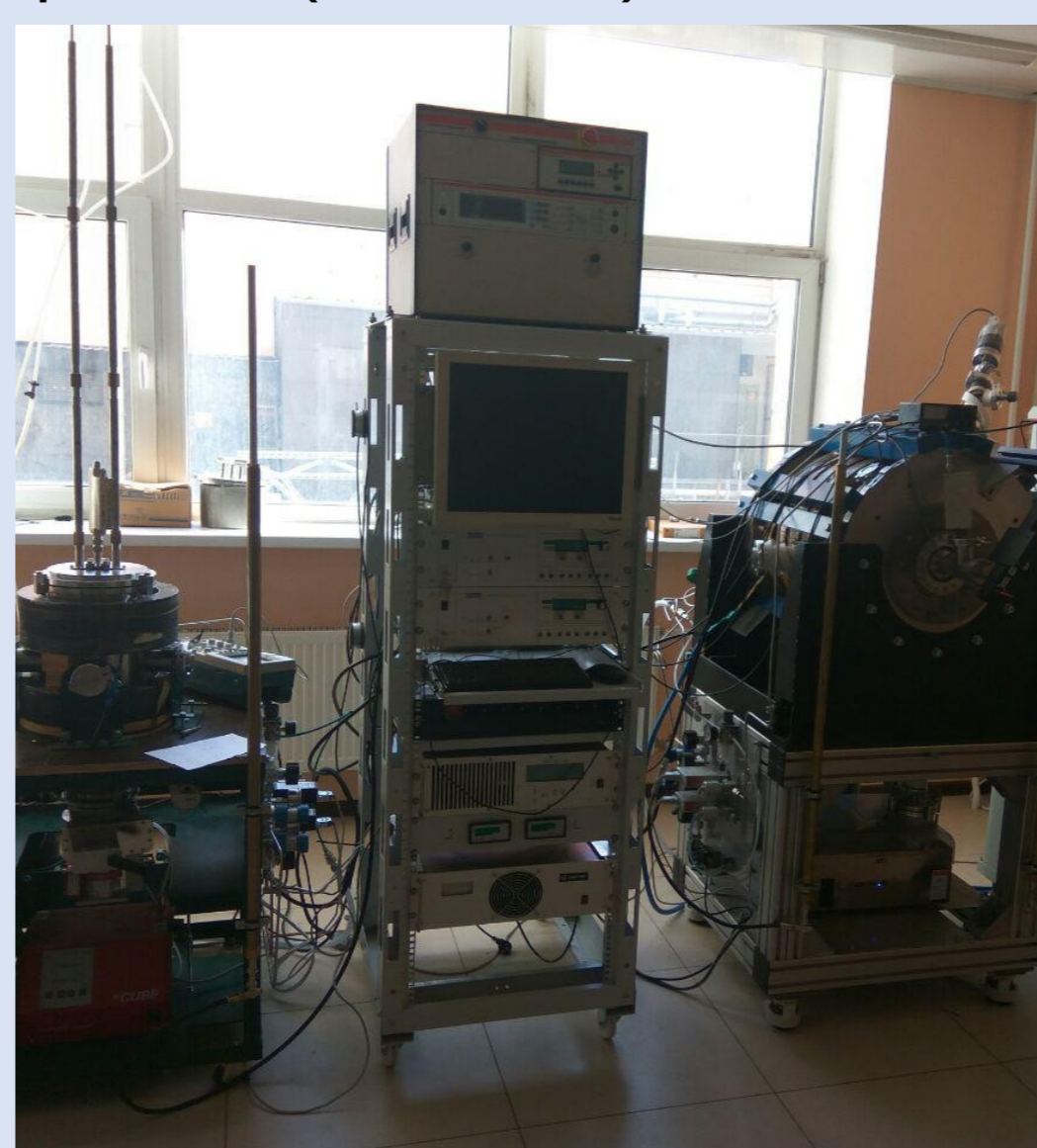
Fig. 4: Experimental setup for research on sputtering and deposition processes in plasma (RF-stand)
