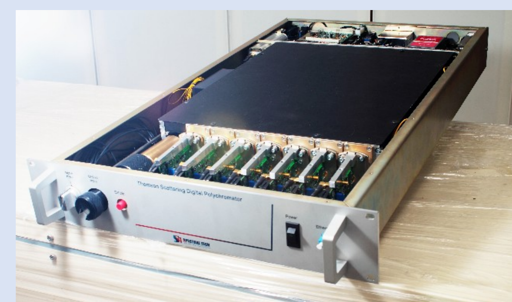
Fig. 3: Digital Thomson scattering polychromator, featuring 8-channel 5GHz ADC
