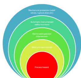
Fig.5. Layer of protection for the W7-X device
