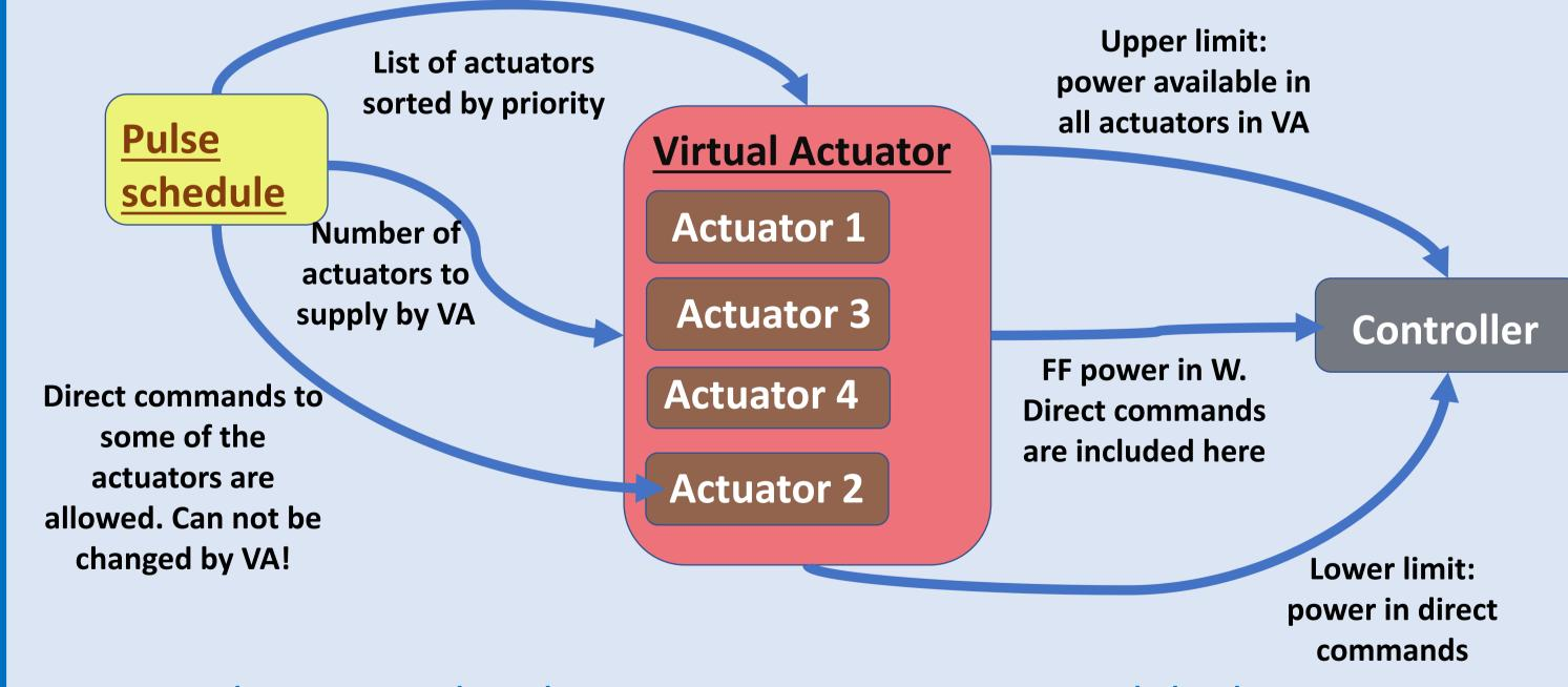
Virtual actuator distributes power to actuators with highest priority
