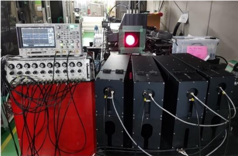
Experimental setup with linear polarizer mounted on the rotation stage with 4-channel APD modules
