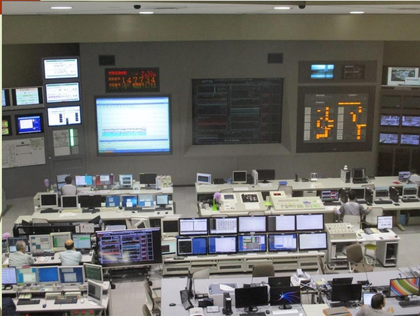
Here is the picture of the central control room. During experiments, MyView2 displays the last results calculated by AutoAna during the repetitive plasma experiments, and it provides the experiment coordinator important information for the following experiment schedule.
