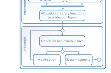
Fig.3. Activity diagram of safety live cycle at W7-X
