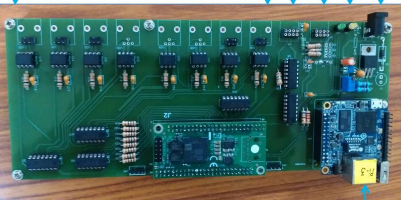
Sub system Module ( slave ) board
